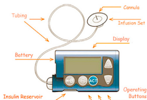
Picture 5: Components of an Insulin Pump
